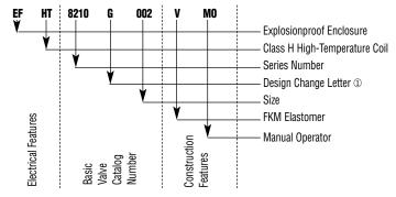
① The Design Change Letter indicates a major design change affecting spare parts kits, rebuild kits, and coils. The correct replacement parts for each change letter are shown in ASCO's Rebuild Kits and Coils Catalog.
